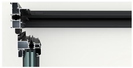
The A82 system is an aesthetic yet sustainable system that utilizes a 3-chamber design, triple seal technology and a multipoint locking system for increased thermal performance, durability and security. Profiles are extruded and thermally broken by means of two continuous polyamide bars 18mm wide. The aluminum alloy is 6063-T5 in accordance with Aluminum Association standards.
