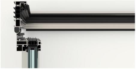
The SlimLine 38 series feature a highly insulated 3-chamber system with ultra-slim profiles for increased thermal characteristics. The solution is available in fixed, turn, and turn-tilt variations with Uf values down to 2.3 W/m²K (1.9 W/m²K for the HI version). The system is suitable for both double and triple glazing options.
